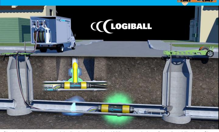
Chemical grouting was originally developed in 1955 as a technique for soil stabilization. Since then, it has been used to stop groundwater infiltration in sewers, manholes, chambers, subways, mines, tunnels and many more underground structures all over the world. Recent studies, combined with over 60 years of experience, show that the original trenchless technology remains the first line of defense and the best long term ROI against groundwater infiltration in structurally sound sewers.
