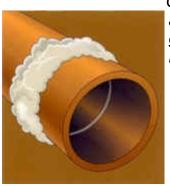
Chemical grout forms a flexible, watertight collar around a pipe joint, thus preventing infiltration. If groundwater pressure increases, the collar will press more tightly against the pipe, sealing even better.
