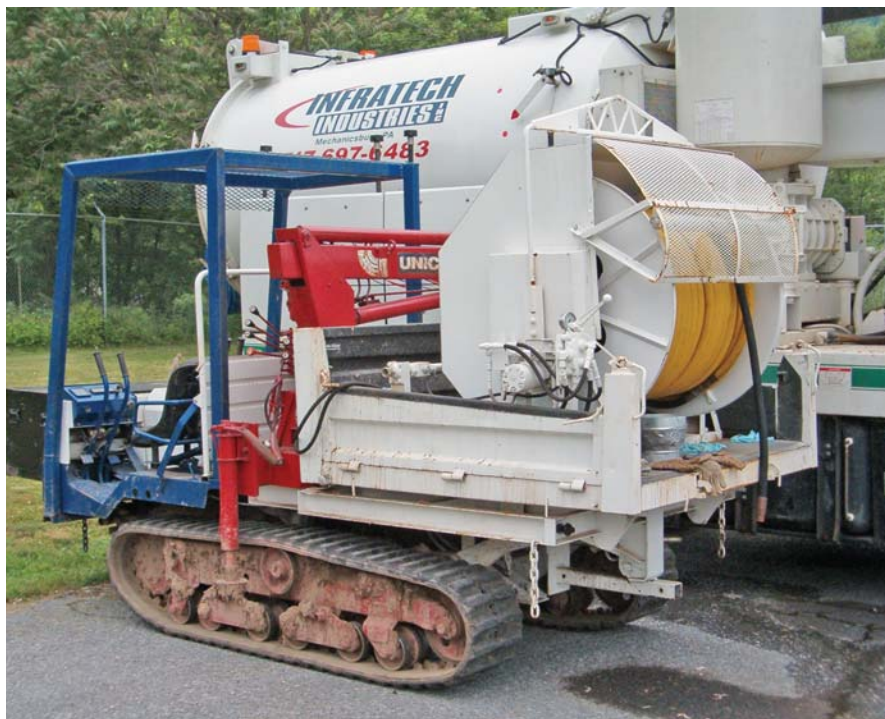
Complete grouting inspection and delivery capability is transported by truck, which carries 500 feet of delivery hose. When further accessibility by truck becomes prohibitive, an additional 500 feet of hose is provided via remote grouter unit.
