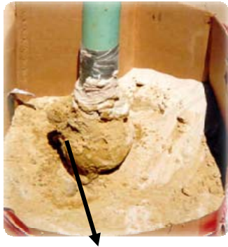
Seal achieved from the outside gelled soil matrix
