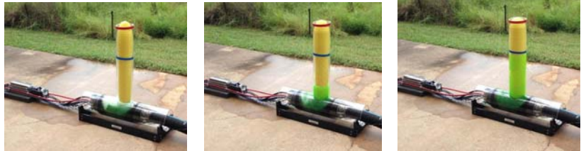
Grout migration from mainline along the lateral bladder
