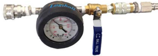
Assembly for setting the cracking pressure of the No-Return Grout valves on the packer. Also used to verify leaks on the packer side of the hoses (vacuum and pressure)
