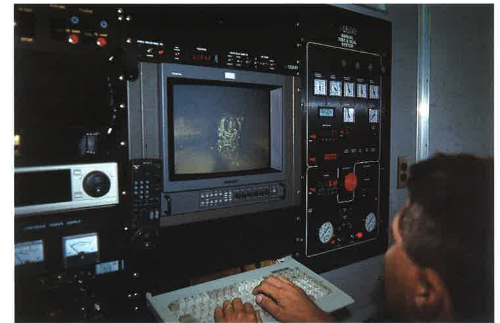
MODERN grout vehicles control and record every aspect of the grouting operation
