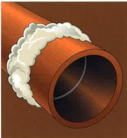
■ CHEMICAL grout forms a flexible, watertight collar around a pipe joint.
