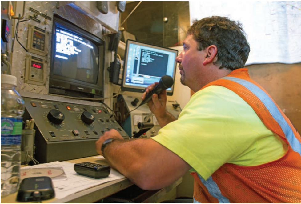
Above: Inside the grout truck, crew leader Charlie Roberts operates Logiball, CUES and Aries equipment, testing and sealing individual laterals. Right: Technician Jason Mahler lubricates the service bladder for the Logiball lateral sealing equipment.
