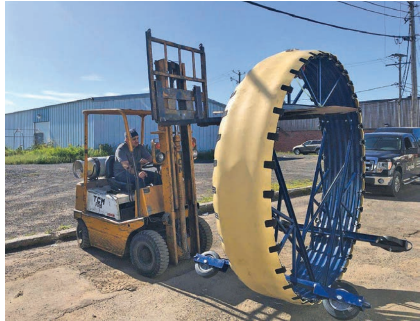
A Logiball team member moves a 96-inch test-and-seal injection packer from one side of the shop to the other.
