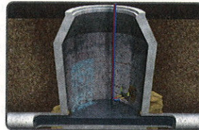
Curtain grouting with wand
