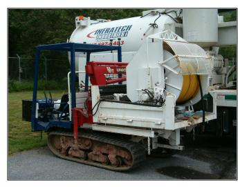
Complete grouting inspection and delivery capability is transported by truck, which carries 500' of delivery hose. When further accessibility by truck becomes prohibitive, an additional 500' of hose is provided via remote grouter unit.
