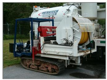
Complete grouting inspection and delivery capability is transported by truck, which carries 500' of delivery hose. When further accessibility by truck becomes prohibitive, an additional 500' of hose is provided via remote grouter unit.
